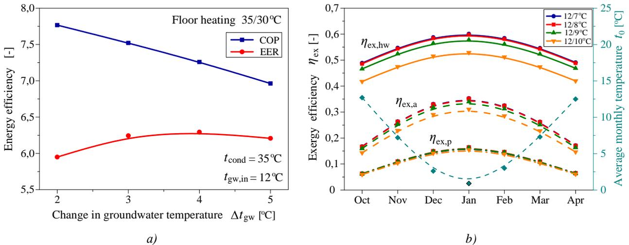
Figure 4. The impact of change in groundwater temperature on: a) COP and EER, b) differently defined exergy efficiencies of GWHP system
