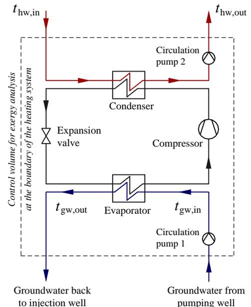
Figure 2. Schematic illustration of the GWHP system
