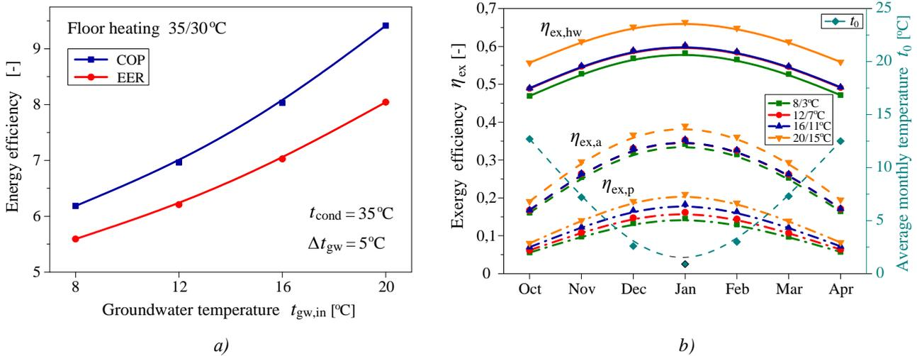
Figure 3. The impact of groundwater temperature on: a) COP and EER, b) differently defined exergy efficiencies of GWHP system
