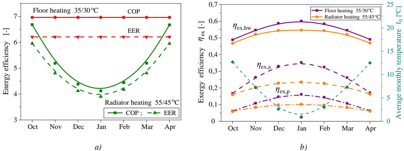
Figure 5. The impact of heating system temperature operation mode on: a) COP and EER, b) differently defined exergy efficiencies of GWHP system (groundwater temperature regime 12/7°C,  $t_{evap}=2^{\circ}\text{C}$ )
