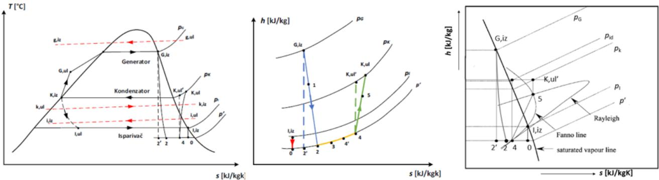
Figure 2. a) Thermodynamic cycle of the ejector refrigeration system for R134a; b)  $h$ - $s$  diagram of ejector working processes; c) Mollier's chart of an ejector.
