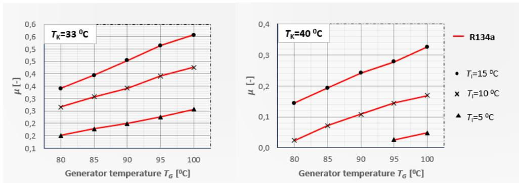
Figure 5. Effect of operating conditions on ejector entrainment ratio for working fluid R134a.
