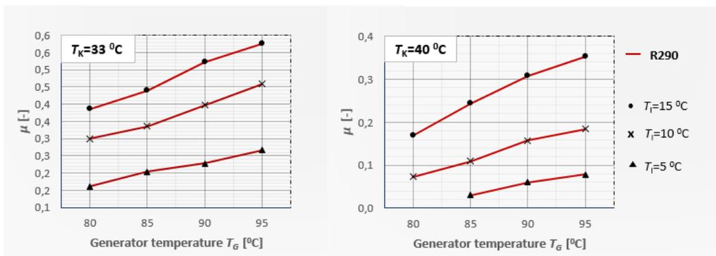
Figure 6. Effect of operating conditions on ejector entrainment ratio for working fluid R290.
