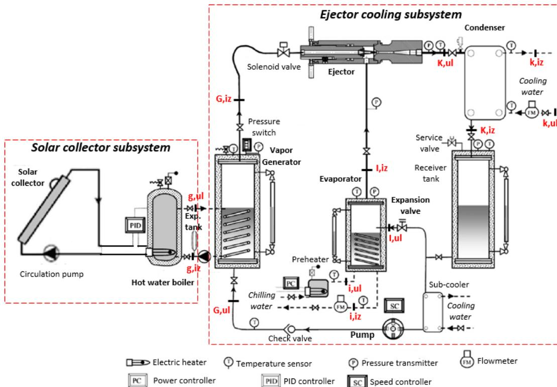
Figure 1. Schematic diagram of solar-assisted ejector cooling system.
