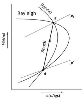
It is assumed that a normal shock wave occurs at the end of constant-area mixing chamber. In this narrow zone, the speed suddenly drops and the pressure surges. As a result, the mixture pressure at ejector outlet is higher than the secondary fluid's initial pressure. Based on the mass conservation, momentum conservation and energy balance equations, the following values are obtained:
