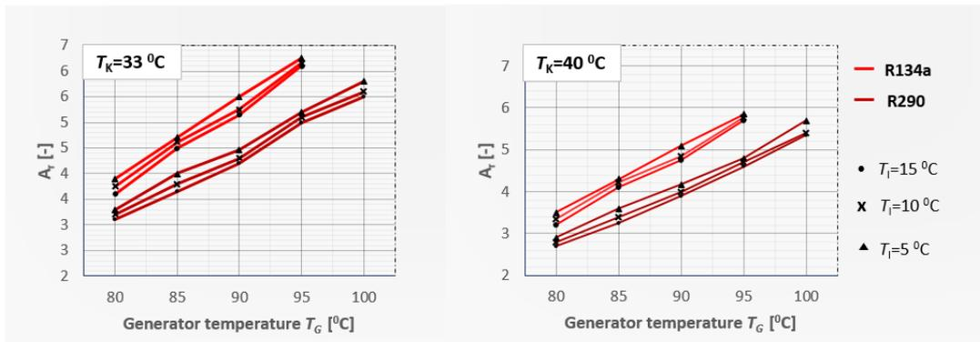
Figure 9. Effect of operating conditions on area ratio for working fluids R134a and R290.
