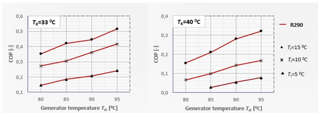
Figure 8. Effect of operating conditions on system COP for working fluid R290.
