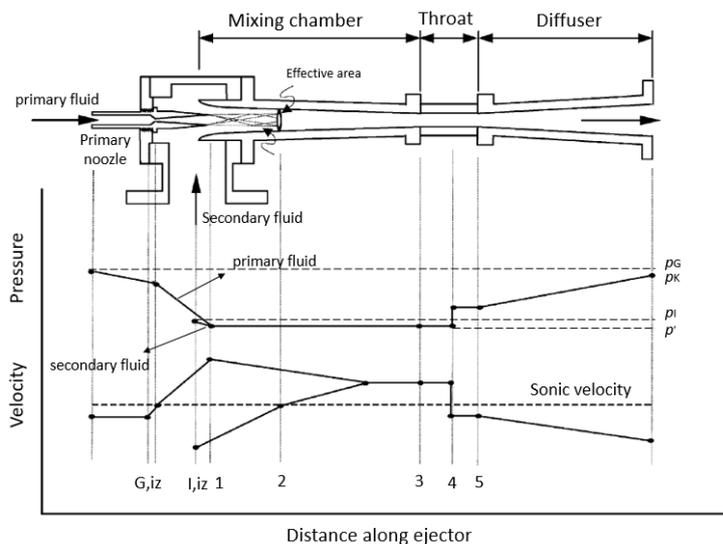
Figure 3. Schematic view and the variation in stream pressure and velocity as a function of location along ejector.
