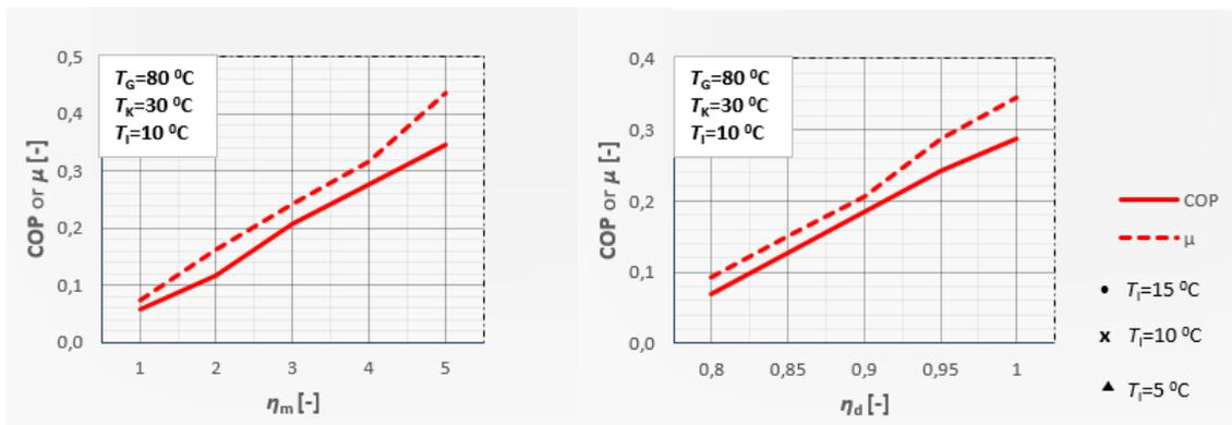
Figure 11. Effect of ejector efficiencies on system COP and entrainment ratio for working fluid R134a.
