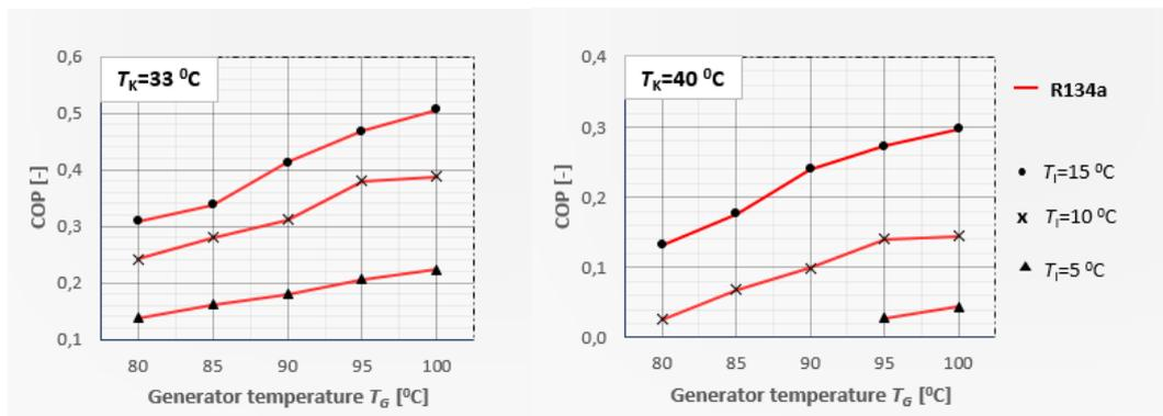
Figure 7. Effect of operating conditions on system COP for working fluid R134a.
