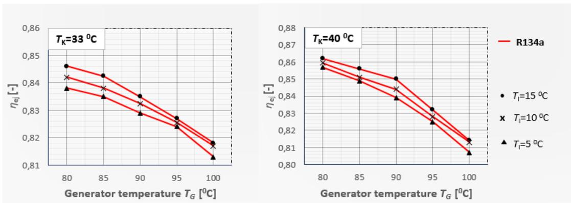
Figure 10. Effect of operating conditions on ejector efficiency for working fluid R134a.
