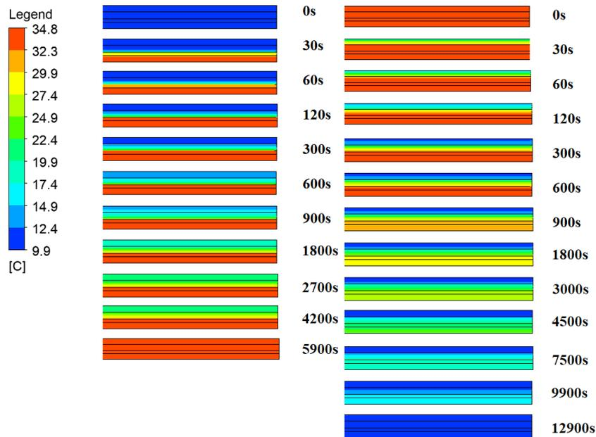
Fig. 8 – PCM integrated electrical heated floor temperature profile throughout the heating and cooling phase
