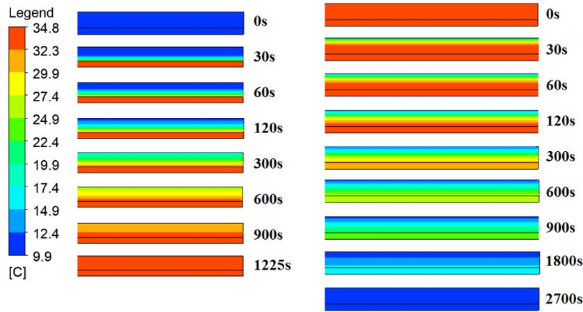
Fig. 7 Electrical heated floor temperature profile throughout the heating and cooling phases
