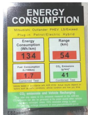
Figure 4. Consumption data for Plug-in hybrid vehicles
