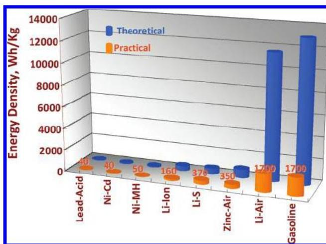
Figure 8. Specific energy of some batteries and gasoline[9]
