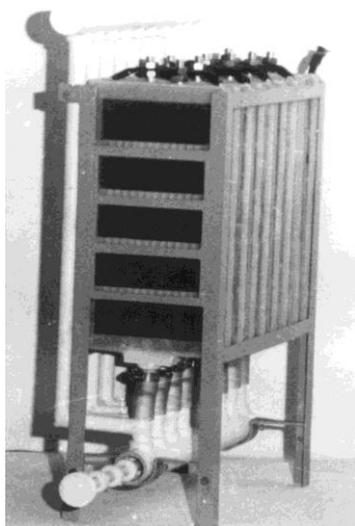
Figure 7. Prototype of the Al-Air battery
