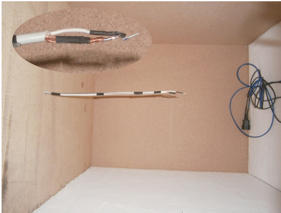
Fig. 6. The interior of the test model - show the position of the PT100 probe
