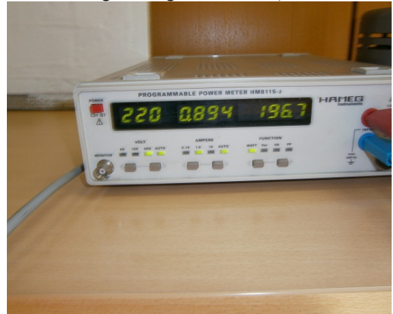
b) Output value of auto-transformer
