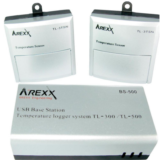
Fig. 4. The sensor for the acquisition of temperature and humidity inside the test chamber
