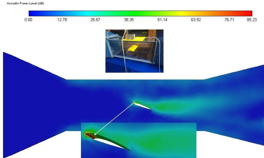
Figure 5: Noise generated by air flow in a straight segment of the duct, noise level at the leading edge
