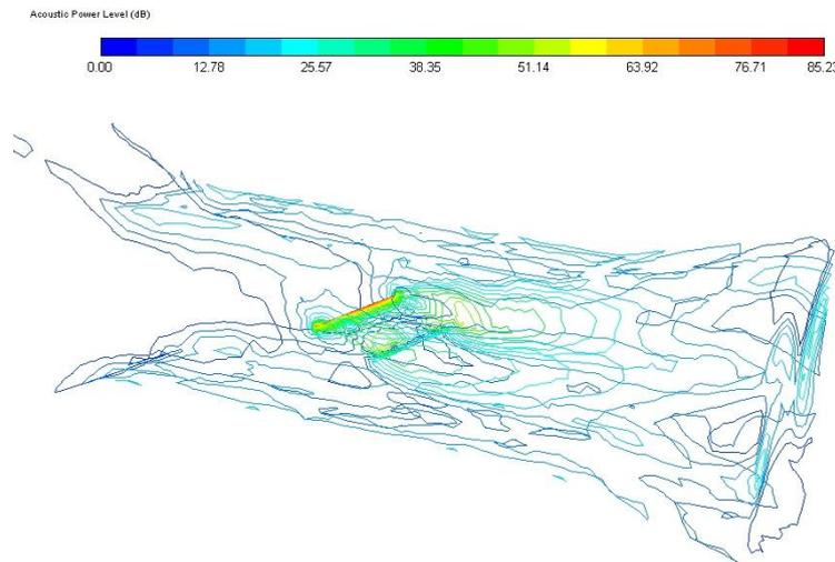
Figure 6: Noise generated by air flow in a straight segment of the duct, 3D Acoustic field
