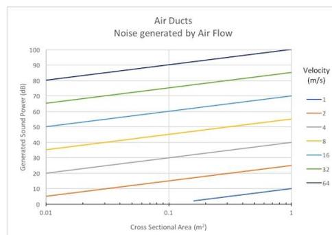
Figure 4: Noise generated by air flow in a straight segment of the duct [4]
