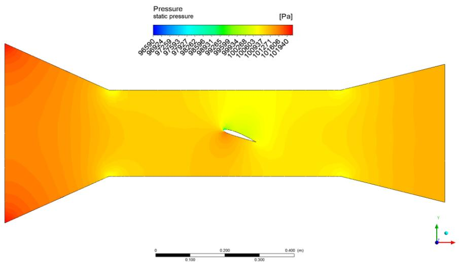
Figure 3: Pressure fields in Computational domain of the straight duct segment of the actively controlled air duct with airfoil vane deflected.
