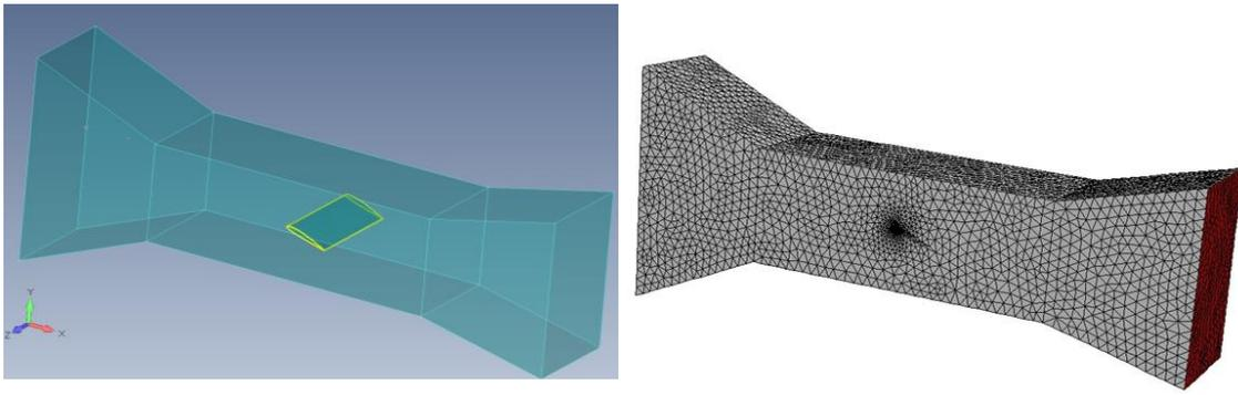
Figure 2: Computational domain of the straight segment of the actively controlled air duct with airfoil vane deflected
