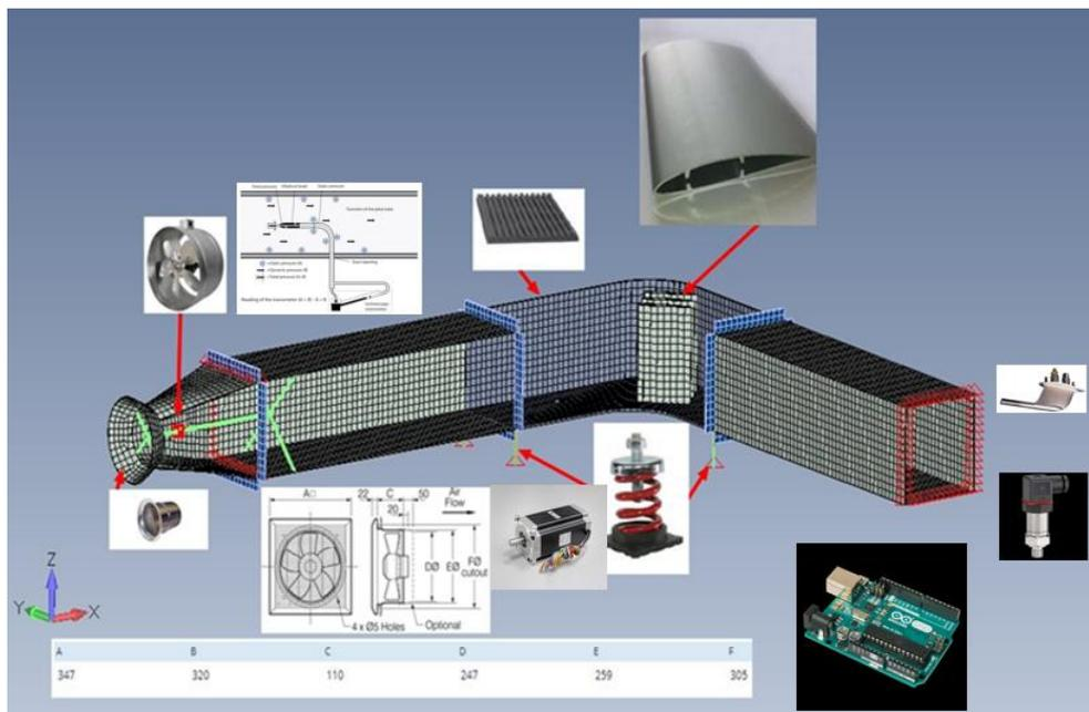
Figure 1: Actively controlled air duct with airfoil vanes-main components schematic
