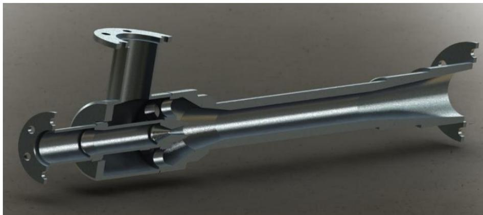
*Figures 6 Cross section view of the ejector flow field*
