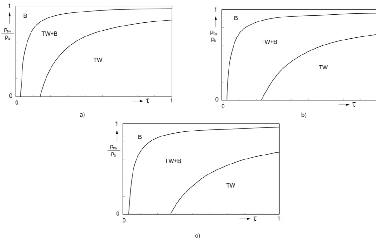
Figure 3 Priority application for the combined low temperature heating system (TW+B), boiler room system (K) and low temperature heating system (TW)
