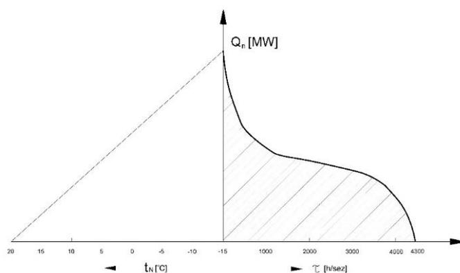
Figure 1 Diagram for heating energy calculation [5]
