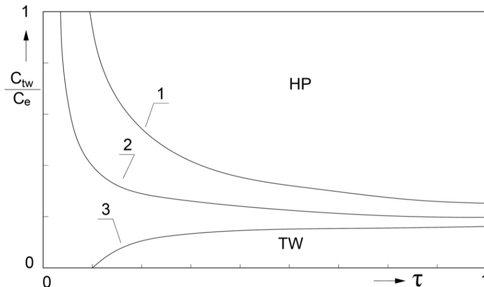
Figure 4 Priority application for the low temperature heating system (TW) and heat pump heating systems (HP)
