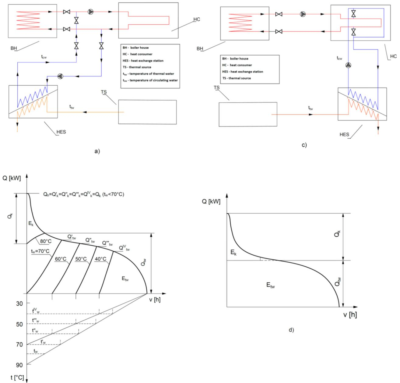
Figure 2 Combined low temperature heating system with single piping circuit (a) and heating diagram (b), combined low temperature heating system with double piping circuit (c) and heating diagram (d)
