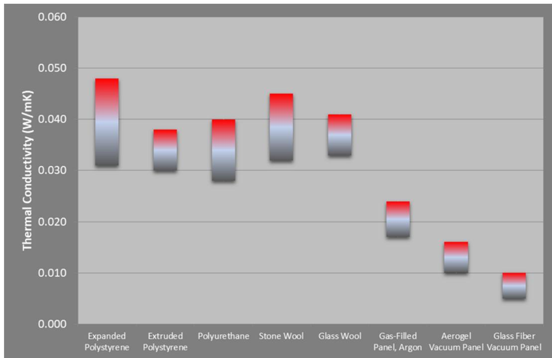
Figure 2: Thermal conductivity values of thermal insulation materials
