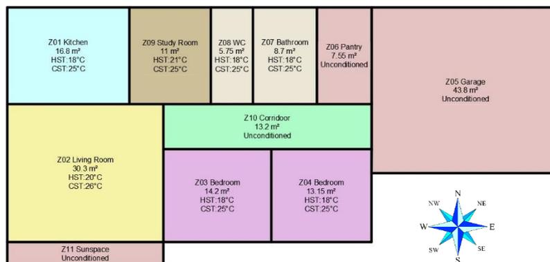
Figure 1: Floor plans and Design Temperatures
