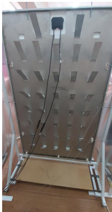
PV panel with wide HP
