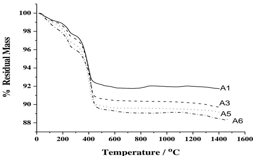
Figure 2. Non-isothermal TG curves of the cordierite mixture mechanochemically activated for different periods of time
