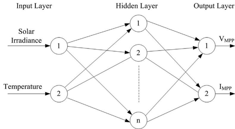
Figure 3. A typical ANN structure for MPPT [2]
