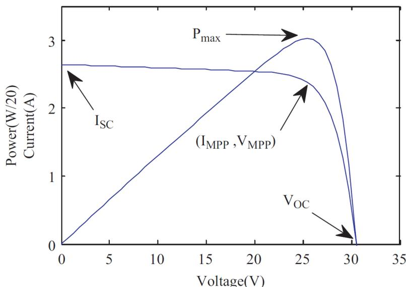
Figure 1. *I-V and P-V characteristics of solar cell [1]*
