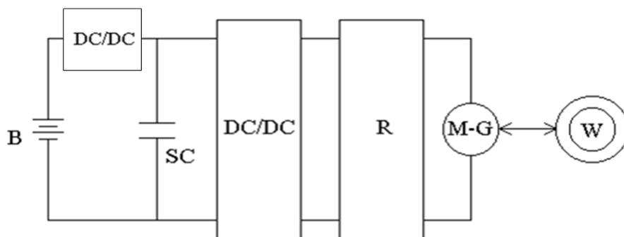
Fig. 2 Scheme of electrical drive vehicle with supercapacitor with possibility for using braking energy; B – one-way voltage source, SC – supercapacitor; DC/DC – direct voltage converter; R – regulator; M-G – engine – generator (depending on working regime; W – drive wheels [2]
