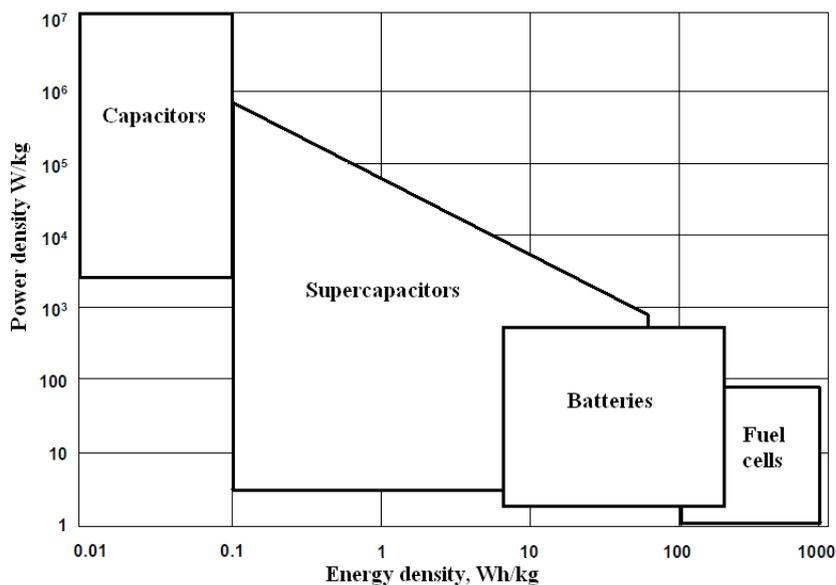
Fig. 1 Area diagram for various energy storage systems [2]
