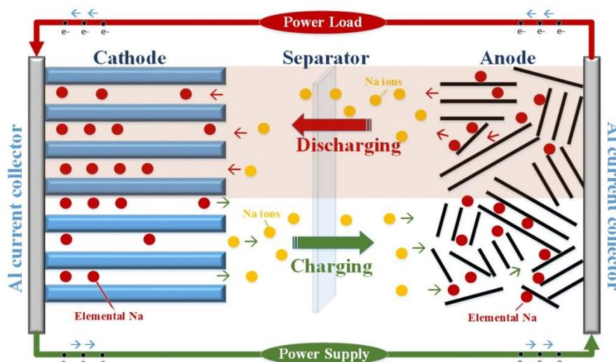
Fig. 6. One concept of battery based on sodium
