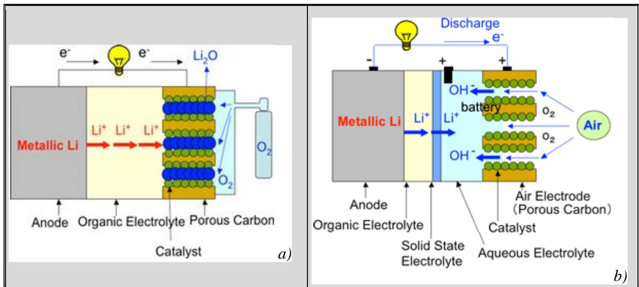
Fig. 4. Configuration of: a) conventional lithium-oxygen battery and b) new lithium-air cell
