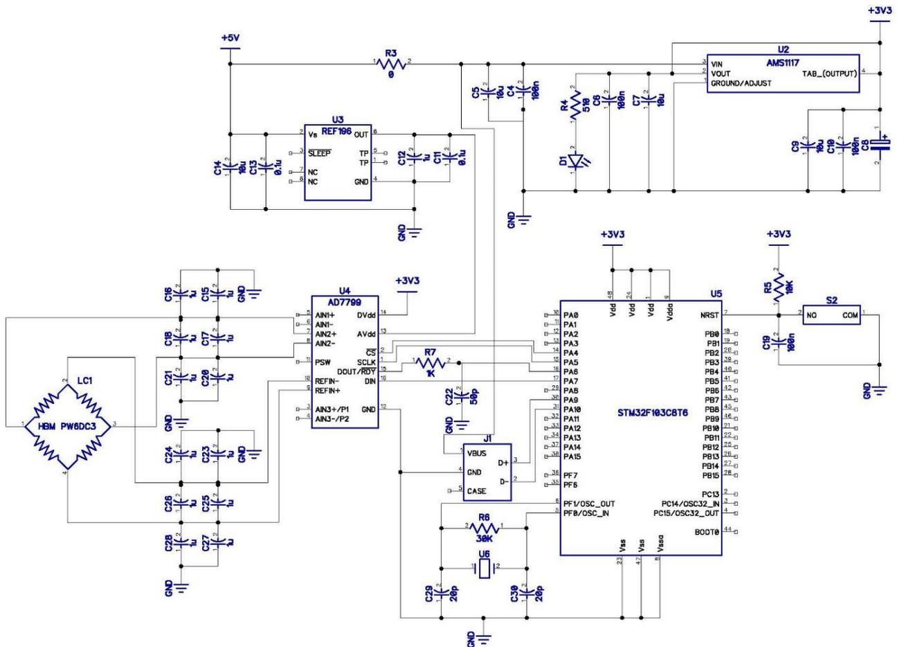
Fig. 2. Electrical schematic diagram of the test bench
