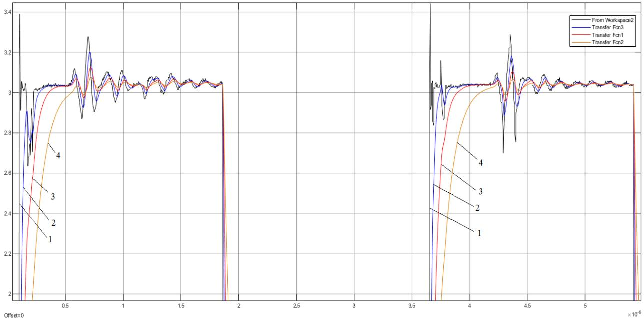
Fig. 7. Plots of transfer functions: 1 - original data from oscilloscope, 2 - transfer function with  $T = 2 \cdot 10^{-8}$ , 3 - transfer function with  $T = 5 \cdot 10^{-8}$ , 4 - transfer function with  $T = 1 \cdot 10^{-7}$
