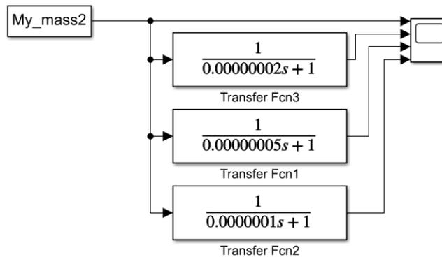
Fig. 6. Transfer function with different time constants T
