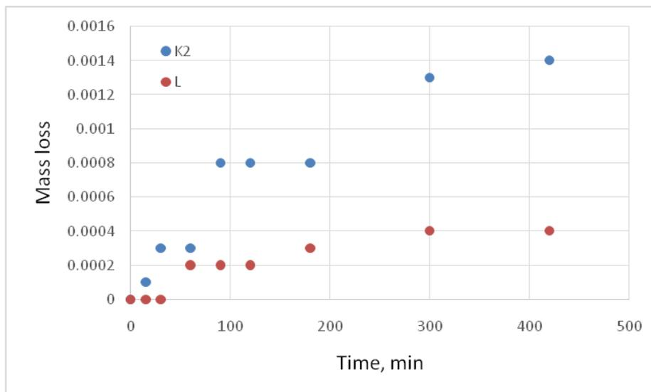
**Figure 5.** Mass loss of CuAlNi shape memory alloy during cavitation testing: L- as-cast samples and K2- quenched samples at 885 °C/60 min H<sub>2</sub>O
