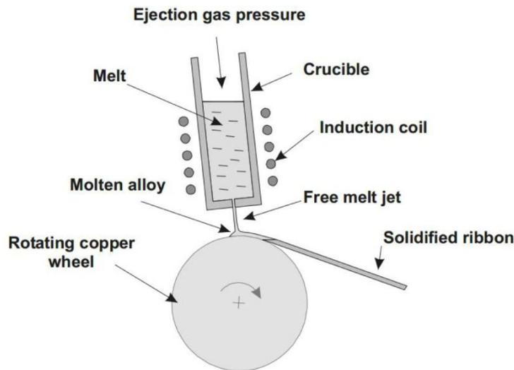
Figure 2. Free jet melt spinner technique [4]
