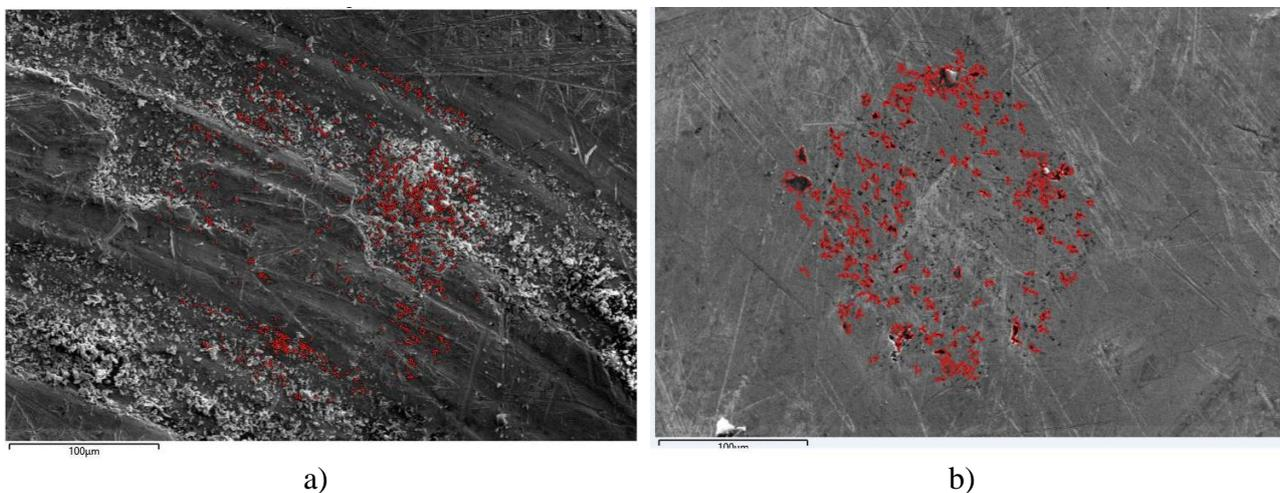
**Figure 6.** SEM images of CuAlNi shape memory alloy in the as-cast state (a) and after solution annealing at 885 °C/60 min H<sub>2</sub>O (b)
