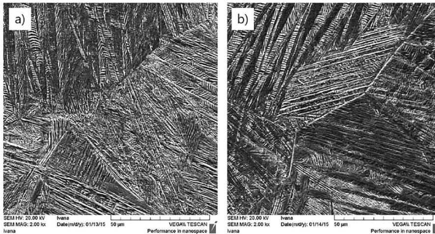
**Figure 4.** SEM images of CuAlNi shape memory alloy: a) as-cast sample (L) and b) quenched sample at 885 °C/60 min H<sub>2</sub>O (K2)
