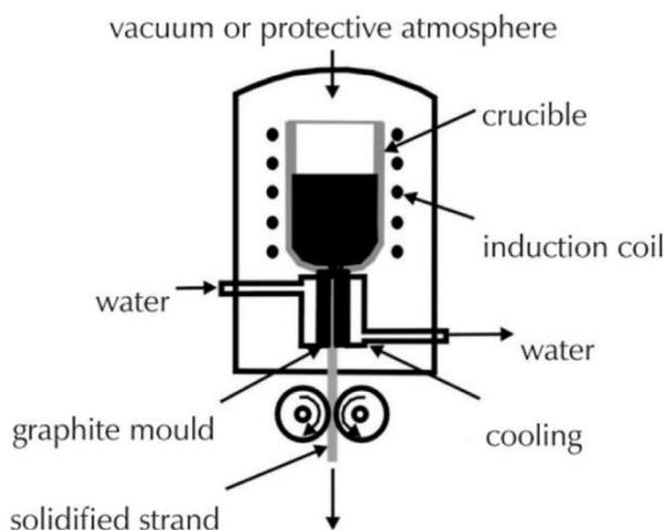
*Figure 1. Casting of CuAlNi alloy by vertical continuous casting technique [7]*
