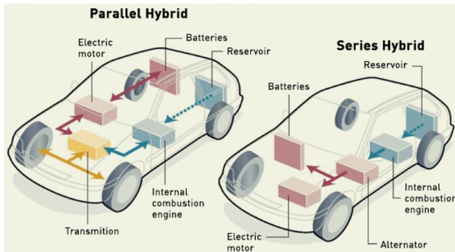
Fig. 2. Concept of two types of hybrid vehicles
