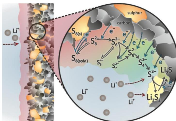
Fig. 3. Part of process in  $\text{Li}/\text{S}_8$  battery [1]
