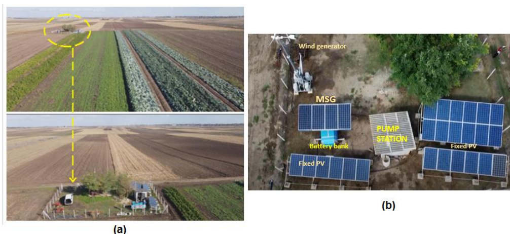
Fig.12. The recording from the drone on the "Smart Land" system and HPSS for irrigation and remote management on the plot "Belegiš"; (a) view of the plot (above) and view of the hybrid power plant based on RES (below, (b) disposition of subsystems of HPSS .
